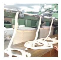
**Figure 4. Drawing Process**
