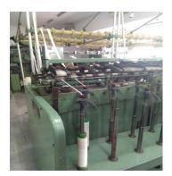
**Figure 5. Roving Process**
